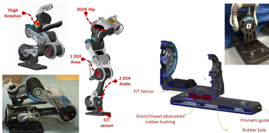
Figure 8. WALK-MAN leg kinematics and foot design
