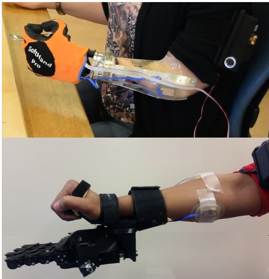
Fig 2. Participants wearing the SoftHand Pro. Top: The SHP attached to a myoelectric socket used by a participant with limb loss. Bottom: The SHP attached to a forearm adapter used by limb-intact participants.
