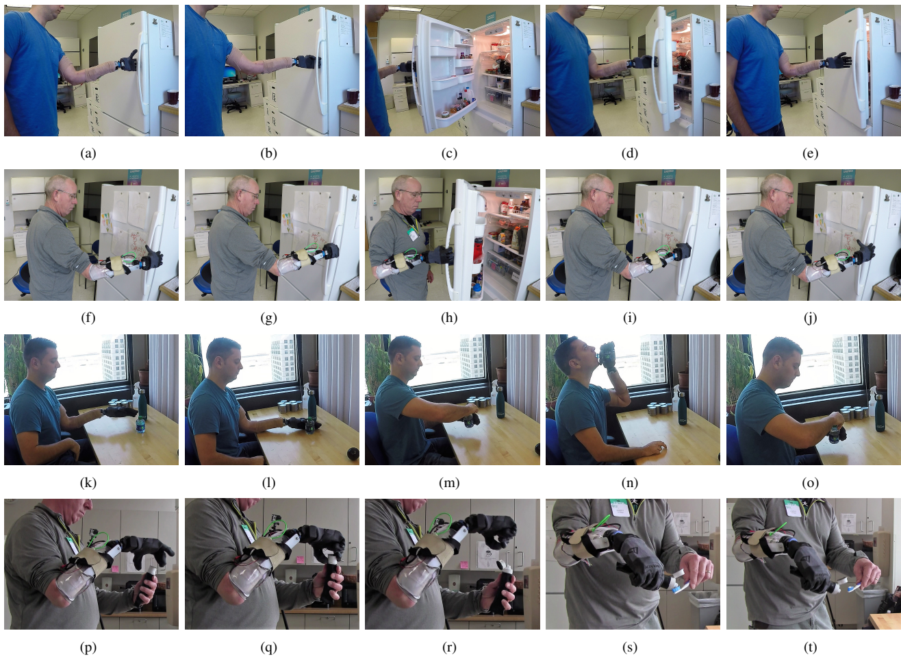
Figure 8: Example of activities performed using the hand-wrist prosthesis: in (a-e) and (f-j) the subjects open and close a fridge door using the wrist movements to follow the door’s trajectory. (k-o) show a bimanual task that involves grasping and opening a water bottle to drink from it and closing it afterwards; wrist flexion is particularly important to ensure correct positioning of the bottle with respect to the subject’s lips when drinking. (p-t) show another bimanual task in which the subject has to open a toothpaste tube and then put some toothpaste on a toothbrush.
