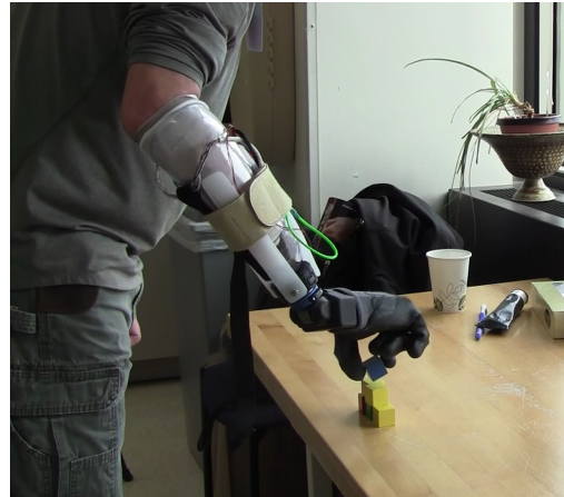
Figure 1: An amputee subject using the hand-wrist prosthesis to stack six wooden blocks in a pyramid. The prosthesis is composed of the SoftHand Pro and the RIC Wrist Flexor.
