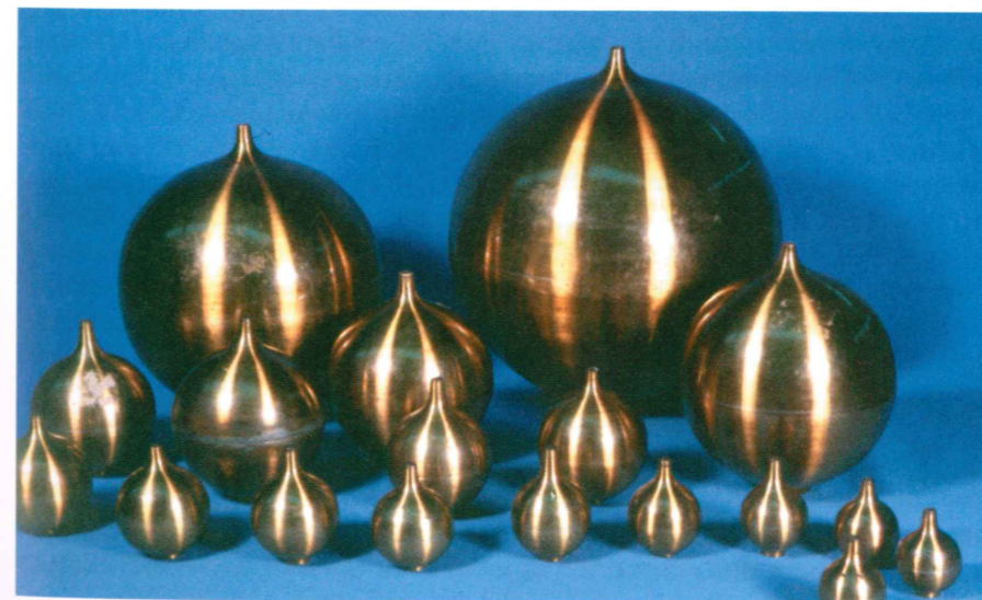
FIGURE 1.23 Helmholtz teamed up with Rudolph Koenig to create these resonators, now known as “Helmholtz resonators.” Each resonator is tuned precisely to a certain frequency of vibration, and when the thin end is held at the ear, listeners can pick out a specific frequency from a complex sound. (Courtesy of Thomas B. Greenslade, Jr.)
