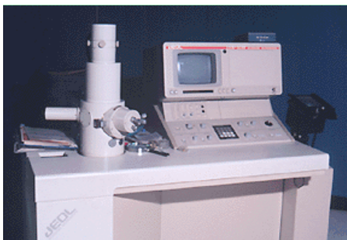
Fig.11 A commercial example of SEM with the analysis chamber on the right.
