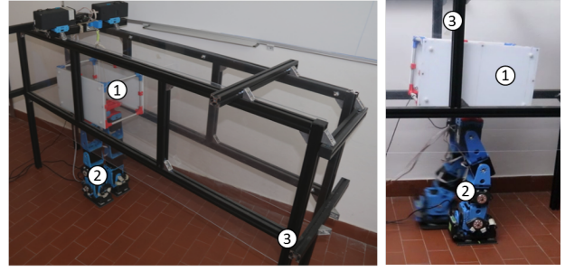
Figure 3 The SoftLegs robot. The system consists of a trunk (1) and two planar legs (2) having 3 DoF each. An external structure (3) constrains the dynamics of the robot to evolve on its sagittal plane.
