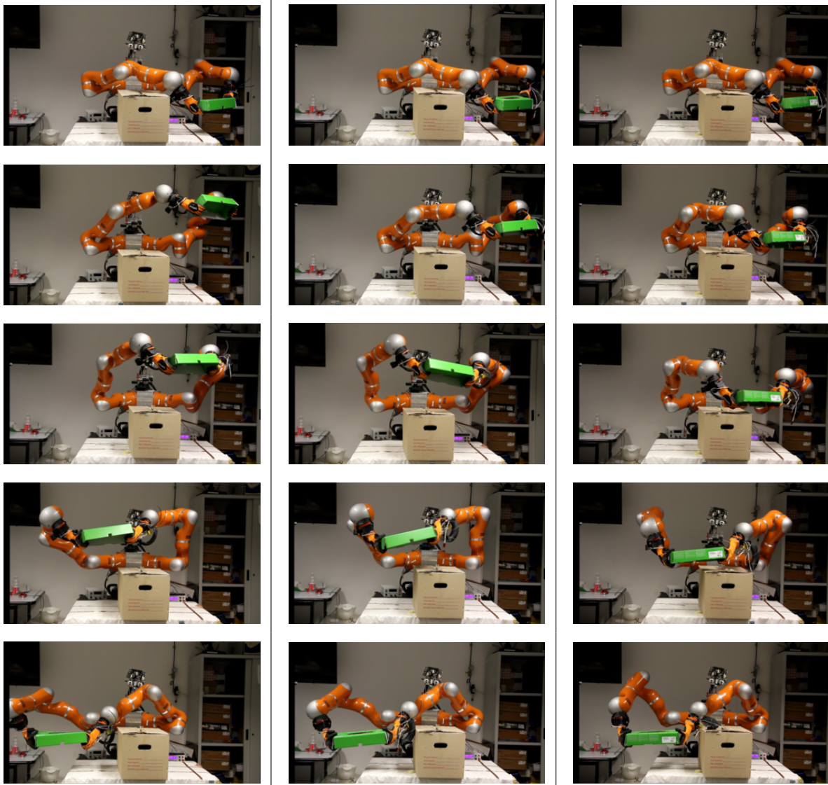
Fig. 9. Snapshots of the experiment using VITO robot. First column shows the first trajectory generated by the planner obtained at 4.32s. Second column is the execution of the trajectory at 7s and the third column is the execution of the trajectory obtained at 10s. It is clear that the trajectory improves with time.
