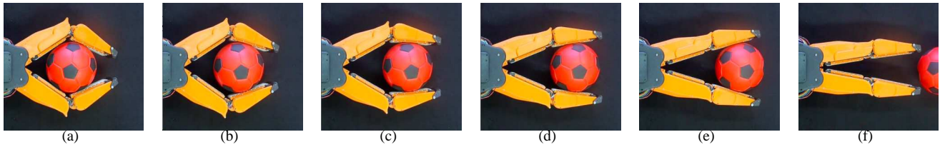
Fig. 12. Object expulsion. A grasped object (a) is completely expelled out of the hand (f) by pushing it with the active surfaces. Adaptability of the under-actuated gripper guarantees grasp stability during the whole movement (b, c, d, e).
