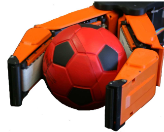
Fig. 1. Prototype of the “Velvet Fingers” smart gripper implemented at the University of Pisa, while grasping a ball.
