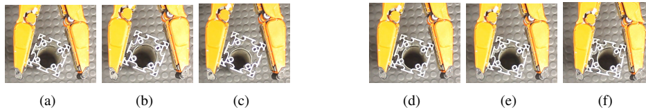
Fig. 13. Different grasp equilibria triggered by different levels of friction. The two sequences, left and right, show the evolution of two grasps starting from same initial conditions but yielding different final configurations thanks to different levels of controlled friction. While on the left sequence high friction ensures stability for the initial grasping configuration, on the right a lower friction level let the grasped object slide in a different configuration.
