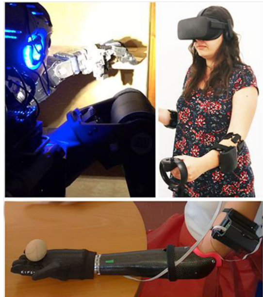
Fig. 1. Picture shows the two envisioned applications of the Stretch Pro: Tele-operation of robot avatars (top panels) and prosthetics (bottom panel). Picture reported in the top-left panel shows the robot Walk-Man during a tele-operated activity in the Amatrice (Italy) village after an earthquake [10].
