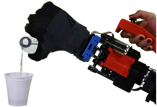
Fig. 1. The two DOFs adaptive under-actuated wrist pouring water.
